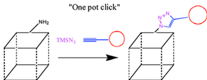
Fig. 19. One-pot, two-step functionalization of an amine-containing MOF, DMOF-NH 2 . Reproduced with permission. Adapted with permission from Ref. [199]. Copyright 2010, American Chemical Society.
